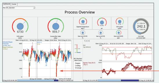
The user can create a versatile Statistical Process Control system to inspect Product Quality at all stages of the production process. The statistical tools available monitor independent samples, grouped data, and automatically generate the most common statistical metrics used in industry. Additional statistical tests can be created by the user through the Python programming language and incorporated into the core software if required.
