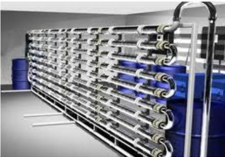
Typical benefits of such systems include waste reduction of 10-15%, energy reduction of 40-70% and solvent hold up that is the order of 10% of the equivalent batch process. A further, major, benefit of these reactors is their ability to manufacture a number of products using a single reactor by rapidly adjusting the operating conditions.
