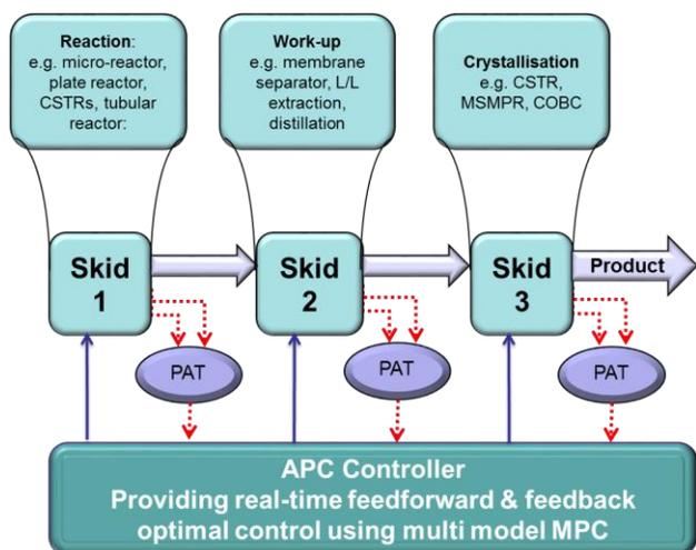
These reactors were supplemented with ancillary units, process instruments and on-line PAT analysers that can be controlled remotely via process automation rather than manual intervention. This set up not only allows the exploitation of the benefits described above, but also gives staff the ability to operate the process remotely, which is of particular interest if the process is hazardous or needs to be operated in a controlled environments such a fume cupboards.
