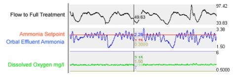
United Utilities and Perceptive Engineering identified an opportunity for further savings, by using ORP (redox) probes and optimizing the MLSS levels in the Orbal stage. In doing so, an **additional 4% of aeration energy was saved**, without compromising the quality of treated water.
